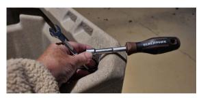
The OptiMizer net is held in place with 4 stainless steel rods, stainless steel fasteners and plastic pieces.
